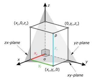
Fig. 1.1: Cartesian Coordinate system illustrating a point p in a three dimensional space. Source: Helmut (2007), Architectural Geometry page 15. Retrieved: 12/12/2022
