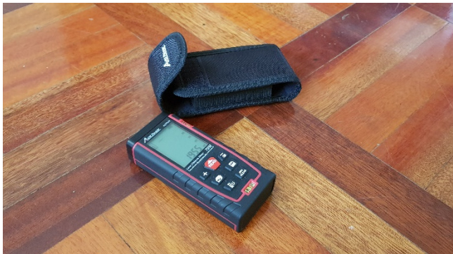
Fig. 4.9 AvidPower Laser Distance Meter (70m) used in physical measurement of spaces.
